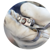
Center groove on knurled thumb wheel prevents wire shift.
