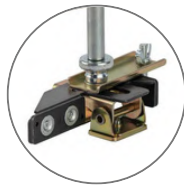
MEH25 features a MagTab base for mounting on square or round tubing or uneven surfaces with additional magnetic planes for mounting stock materials.
