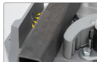
Magnets in the walls instantly hold pipes, tubes, angle iron, or metal plates in position.
