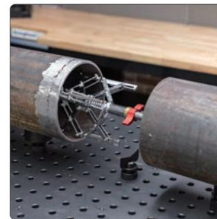
Used for Pipe Butt-welding
