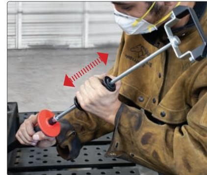
Adding the extension and handle (ASRX48) extends its applications to scrapping/chiseling spots on the floor or on high location.
